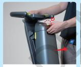
Press the unlock button(D),  $\,$  pull out the solution tank from main body.
