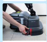
Hold the lift handles on both sides of the squeegee, lift up once to raise the squeegee, lift up again to put down the squeegee.
