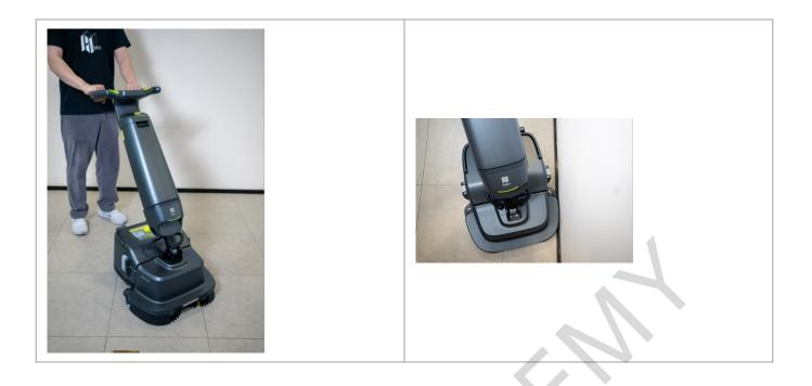
When using the "Soak" and "Brush max" modes to clean unremovable stains, you can raise the squeegee to increase its cleaning power. Put your hands underneath squeegee lift handle and lift them upward or push down to lower the squeegee.
