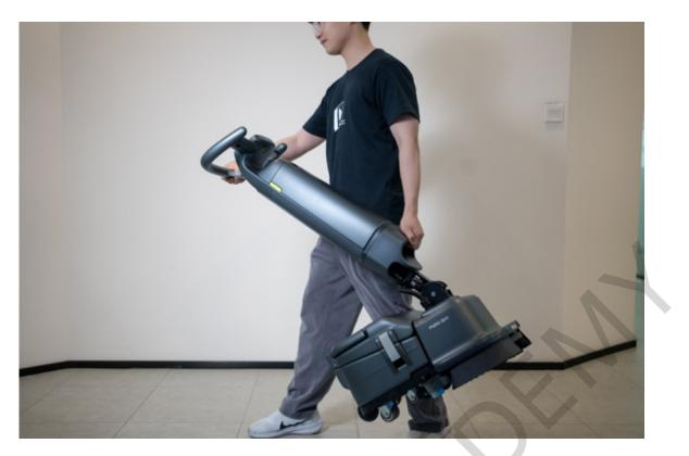
When carrying the device, it is recommended to refer to the pic. For inconvenience, solution tank and the recovery tank can be dismantled to reduce the weight.
