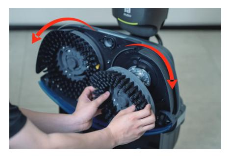
Take the disc brushes (left and right undefined), and in the storage position of the device, install the disc brushes by aligning them with the chassis disc brush mounts and rotate outward to install.
