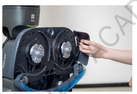
Align the two fixing clips on the left and right splash guards with the card holes and press to fit.
