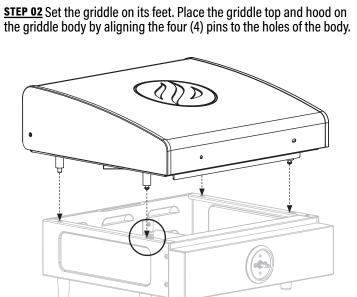
Make sure the front pins are fully seated in the holes, then push the griddle top back to lock the griddle in place.
