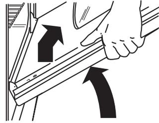
3. Pull door straight up, then toward you. Do not remove hinge pins until the door is replaced on the range.
