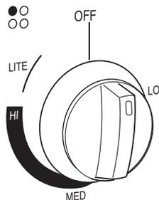
3. Turn control knob to the "HI" position after burner lights.
