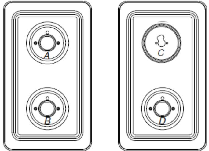
A. Standard burner - Propane gas orifice spud number 88
