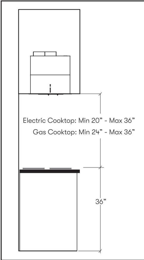
A minimum of 6" round vertical or horizontal duct must be used to maintain maximum air flow efficiency.
