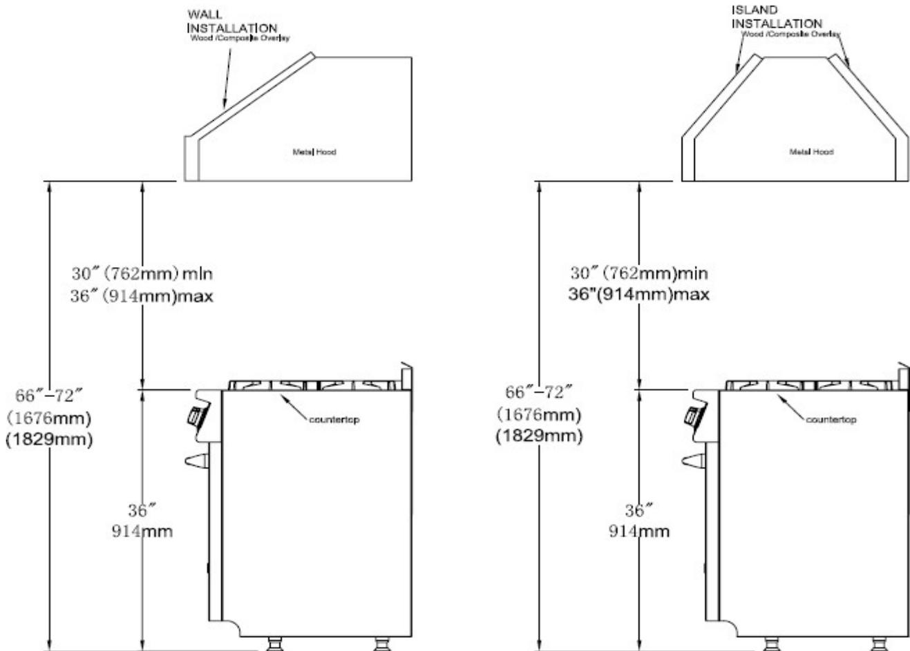
The bottom of the hood should be 30" min. to 36" above the counter top. This would typically result in the bottom of the hood being 66" to 72" above the floor. These dimensions provide safe and efficient operation of the hood.
