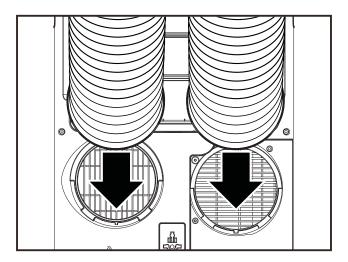
2. Insert window panels B and C to each end of the main panel A with the exhaust and intake port cut outs. Adjust the length of the window panel kit by using the screws and nuts mounted on the two ends of the main panel A.
