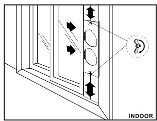
4. Insert the other end of exhaust and intake hose assembly with the hose connector to the window kit onto the window panel kit and turn counterclockwise to secure.
