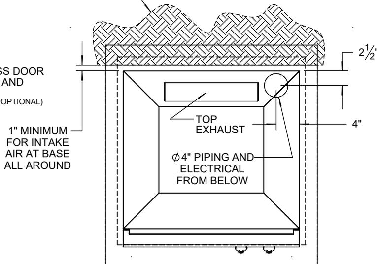
REFER TO AXE-PZA MANUAL FOR PROPER CLEARANCE TO NON-COMBUSTIBLE MATERIALS AND OTHER CONSTRUCTION
