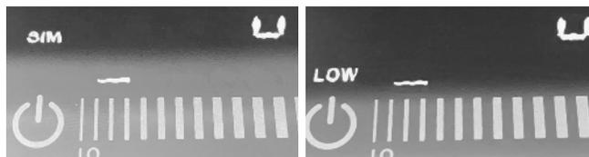
**Deactivate Simmer** by switching to a higher level, lift and touch the **Heating Level Control Sweep** to the right until the desired level is displayed.
