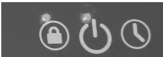
**To Unlock the cooktop** touch the lock graphic. An audible beep will be heard and the light above the lock graphic will go out. The cooktop is now unlocked and all functions operate.
