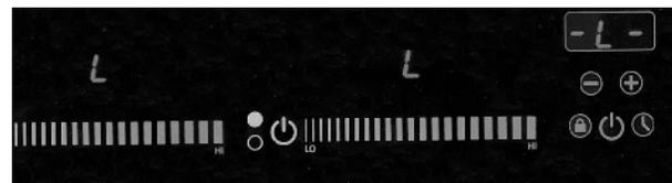
**To Turn Off the Child Lock** simultaneously touch and hold the lock and clock graphic. An audible beep will be heard and the cooktop will be unlocked.
