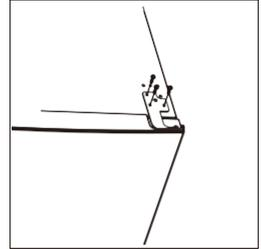
2. Remove the pin with a screwdriver and flip the hinge bracket. Then refit the pin to the hinge bracket.
