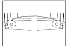
9. Disassemble the right hinge, find the right bottom hinge from the spare parts bag, and fix it.
