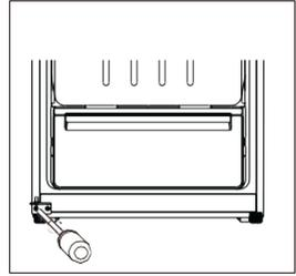
11. Reverse the direction of the middle hinge by 180°, then transfer it to the left property position. Place the middle hinge pin in the upper hole of the lower door, then tighten the bolts.
