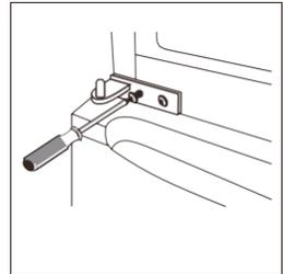
12. Place the upper door back onto the unit. Ensure the door is aligned horizontally and vertically so that the seal is closed on all sides before finally tightening the top hinge. Then insert the top hinge and screw it to the top of the unit and then the affix hinge cover (in the accessory bag) by using the screws.
