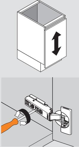
On non-cam mounting plates, loosen screws, adjust door and retighten screws.
