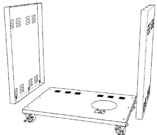
5. Attach Bottom Back Panel - The bottom back panel first gets secured to the Bottom Cart Panel with screws (The bottom of the panel has openings for screws to go through, see diagram). The amount of screws used vary by the size of the grill cart you are assembling. **Attach but do not tighten.** Next secure the Bottom Back Panel to the right and left side panels. Three screws get used per side. **Attach but do not tighten.**
