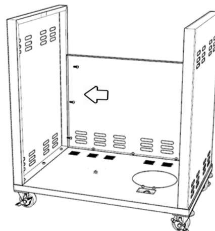
6. Attach Upper Back Panel - This panel gets attached to the left and right panel with 2 screws per side. **Attach but do not tighten.** Attach the Tank Interference Bracket - (Not included for a 3 burner cart model). This pieces are to intended interfere with a second LP tank being stored inside the grill cart which is not permitted. Using 4 screws, attach and tighten the Tank Interference bracket to the 4 nutserts adjacent to the large circular cutout for the LP tank (see figure D)
