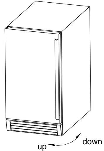
1. Place a carpenter's level on top of the unit to see if the ice maker is level from front to back and side to side.
