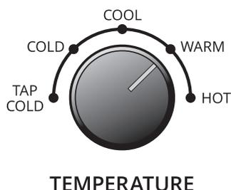
Once you select a cycle, select the desired wash temperature by turning the Temperature knob to the appropriate setting based on your load. All rinses are tap cold.
