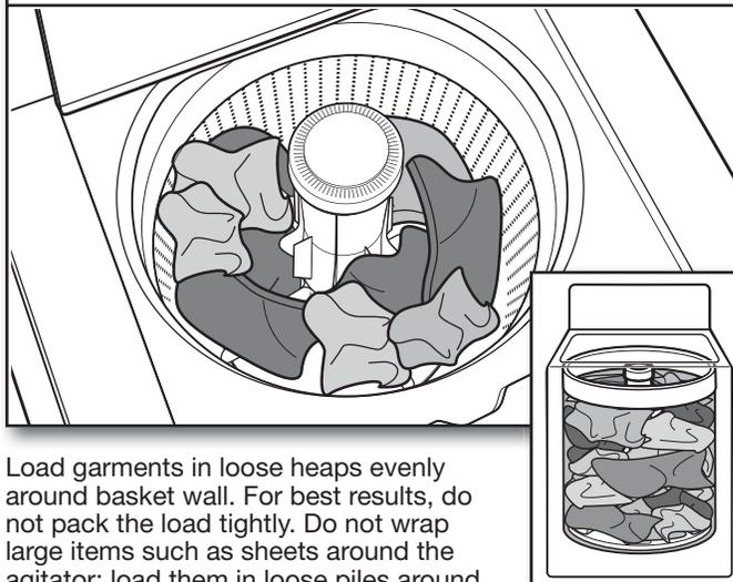
Load garments in loose heaps evenly around basket wall. For best results, do not pack the load tightly. Do not wrap large items such as sheets around the agitator; load them in loose piles around the sides of the basket. Try mixing different sized items to reduce tangling.
