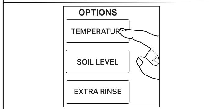
Once you select a cycle, select the desired wash temperature by repeatedly pressing the Temperature button to select the appropriate setting based on your load. All rinses are tap cold.
