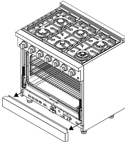
5. Remove the kick plate by unscrewing 3 screws securing it to the oven — 2 on each side of the top lip and 1 in the middle, as shown above. Then, lift up and pull out of the holes on each side to remove the kick plate. To install a new kick plate, position the kick plate into the holes on each side of the range and then replace the same 3 screws.
