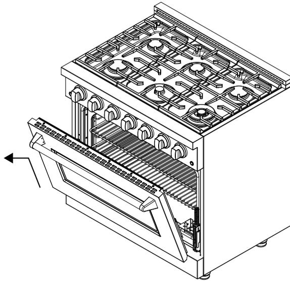
4. Lift the door up and pull it toward you, releasing it from the hinge receivers, as outlined in the image above. The door will gently detach from the oven. If the door does not easily detach from the oven, do not apply force. Make sure the levers are unlocked. To install a new door, follow the reverse of steps 1–4.
