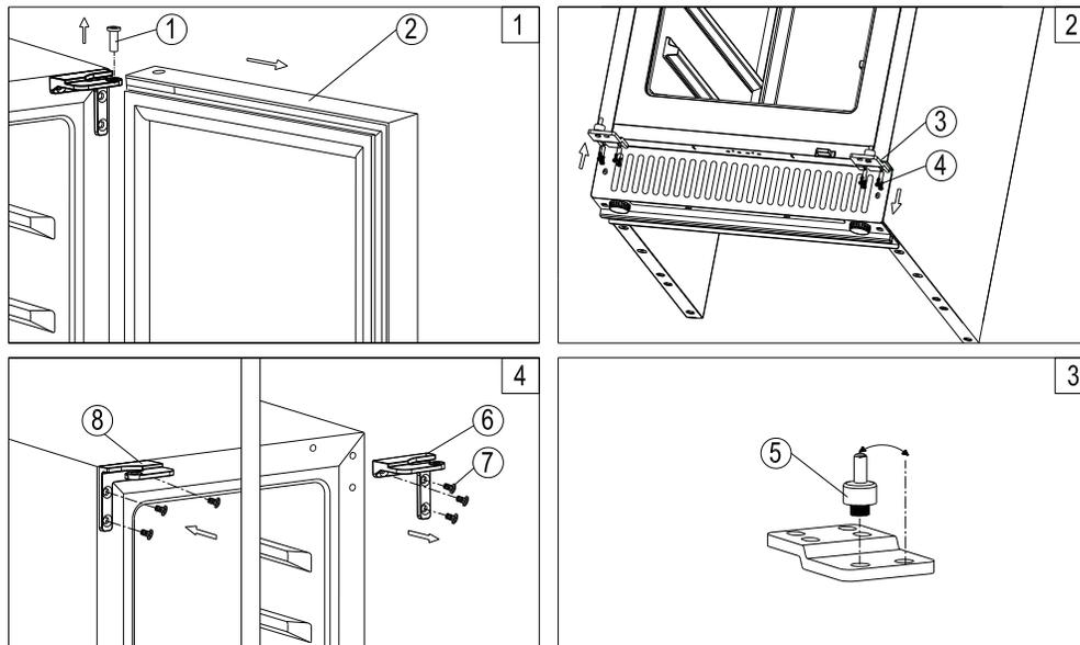
1. Unscrew the top hinge pin 1 and then remove the door 2. Be careful to hold the door firmly after removing the hinge pin and place the door on a padded surface to avoid the risk of damage. Then remove the right top hinge 6. (Figs. 1 & 4)
