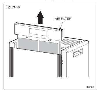
STEP 2. Clean the air filter with a vacuum cleaner or wash it with clean water and dry with a dry cloth (See Figure 26).
