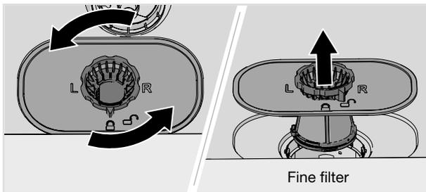
1. Turn the lock ring counterclockwise and lift the fine filter straight up.
