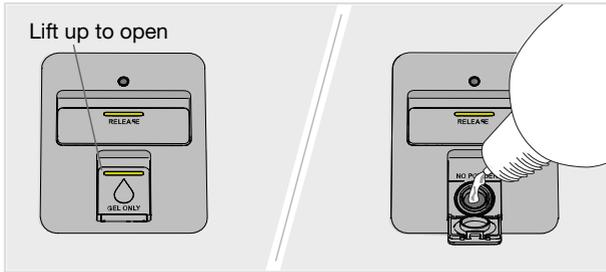
1. Open the lid of the automatic dosing compartment for dishwasher detergent gel.
