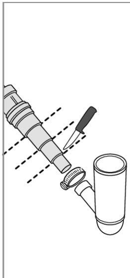
The drain hose can also be connected to a connection nipple on the sink unit's water trap. The connection nipple must have an internal diameter of at least 1/2" (14 mm).
