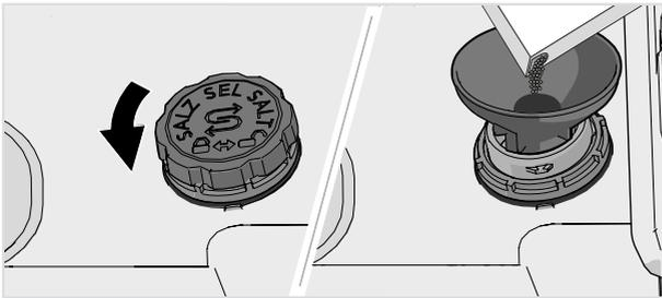
1. Remove the salt compartment lid by turning it counterclockwise.
