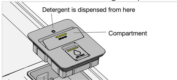
1. The compartment can be lifted out for cleaning and refilling.
