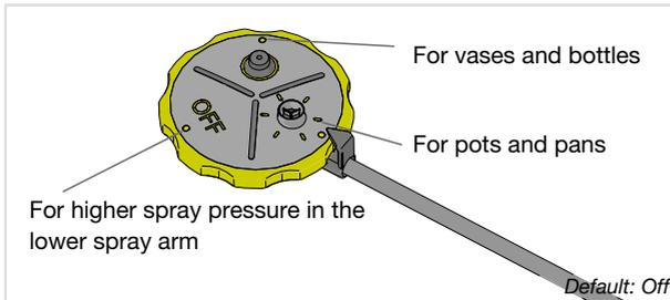
Leave the power zones open if you want an increased water flow where, for example, you have placed pots and pans or vases and bottles. Turn the dishwasher's power zones off if you want greater spray pressure in the lower spray arm.
