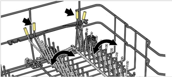
At the back of the right side of the lower basket, the plate supports can be pushed together to provide more space for, say, stoneware or a large pan.
