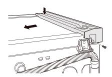
Place the appliance on top of the washer, fitting the dryer feet into the side brackets as illustrated. Avoid finger injuries; do not allow fingers to be pinched between the washer and the appliance. Slowly slide the appliance toward the back of the washer until the side bracket stoppers catch the dryer feet.
