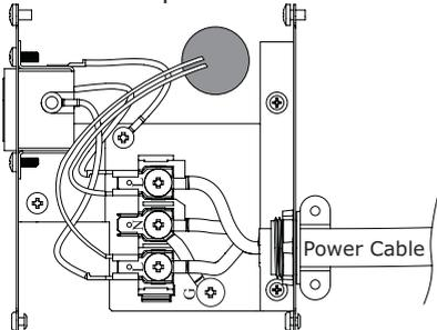
The dryer is now ready to be plugged into the 3-wire receptacle of the proper rating.
