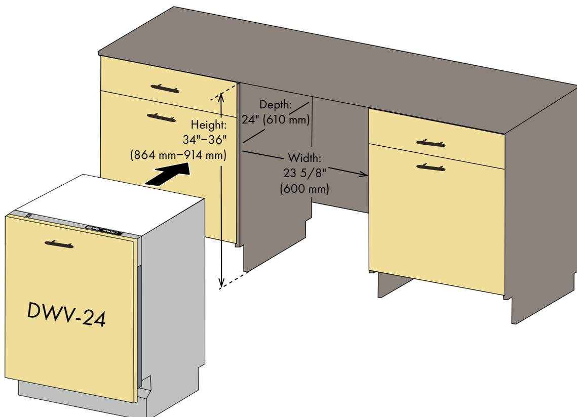
**NOTE:** Since kitchen layouts vary, ZLINE recommends consulting with a professional installer to verify cabinet dimensions before installing the appliance.
