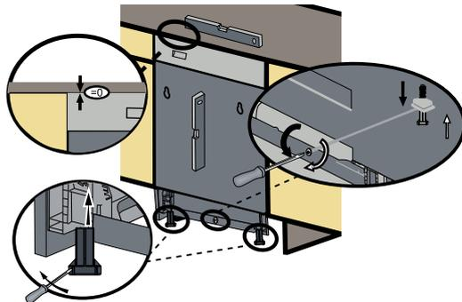
If the height is above 34 1/8" (867 mm), use the long leg supports as shown in the figure above.
