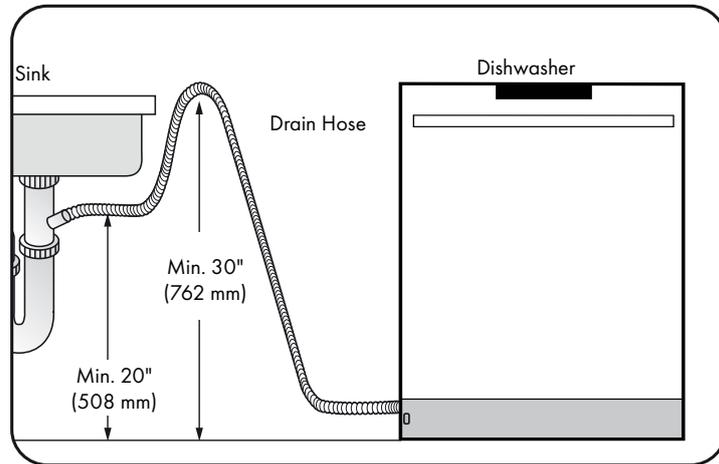
6. When drilling a hole for the drain hose through an adjacent cabinet panel, use caution to not cause damage to the drain hose by any sharp edges of the hole. If the panel is wood, be sure to sand any rough edges before routing the drain hose through. If the panel is metal, be sure to protect the drain hose by using a suitable edge protector or grommet (not supplied) made for this purpose by the manufacturer.
