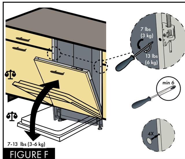
9. After adjusting the door tension, the holes can be covered with the four provided adhesive hole covers (f).
