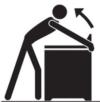
To check if the anti-tip bracket is installed properly, use both arms and grasp the back edge of the range. Carefully attempt to tilt the range forward. When properly installed, the range should not tilt forward.
