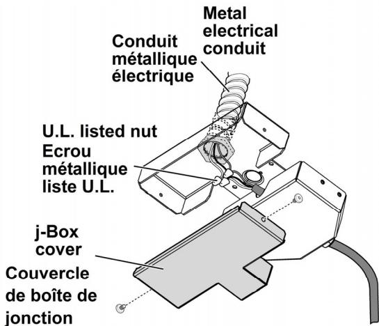
Run 3 wires; black, white and green ,according to the National Electrical Code and local codes and ordinances, in 1/2" conduit from service panel to junction box. Connect black wire from service panel to black or red in junction box, white to white and green to green-yellow.
