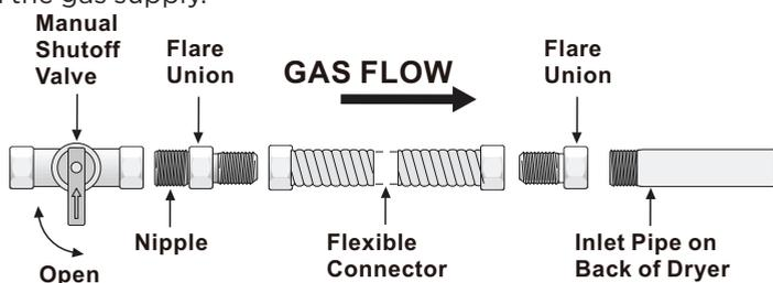
All connections must be wrench-tightened
