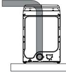
Clean all old ducts before installing your new dryer. Be sure the vent flap opens and closes freely. Inspect and clean the exhaust system annually.
