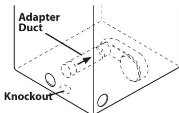
3. Insert the 4 inch (10.2cm) elbow through the rear opening and attach it onto the adapter duct. Be sure that the male end of the elbow faces down through hole in the bottom of the dryer. Secure in place with aluminum tape. Attach aluminum tape to the back of the dryer.
