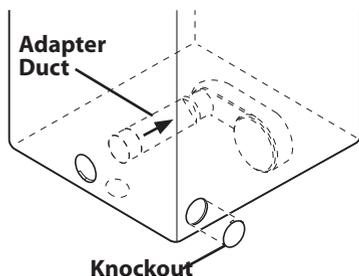
3. Preassemble a 4 inch (10.2cm) elbow to the next 4 inch (10.2cm) duct section, and secure all joints with aluminum tape. Be sure that the male end of the elbow faces AWAY from the dryer. Insert the elbow/duct assembly through the side opening and attach it onto the adapter duct. Secure in place with aluminum tape. Be sure that the male end of the duct protrudes 1.5 inches (3.8cm) to connect the remaining ductwork. Attach aluminum tape to the back of the dryer.
