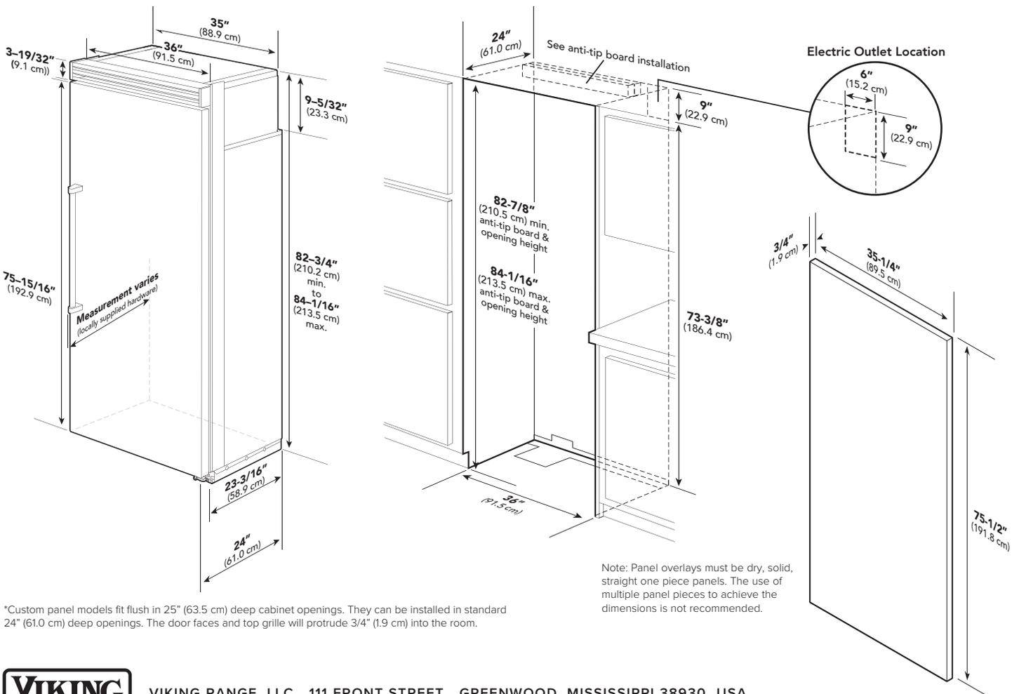
\*Custom panel models fit flush in 25" (63.5 cm) deep cabinet openings. They can be installed in standard 24" (61.0 cm) deep openings. The door faces and top grille will protrude 3/4" (1.9 cm) into the room.
