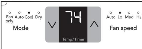
Note: The fan speed can be selected among four settings: Auto, Lo(Low), Med(Medium) and Hi(High), unless the unit runs in "Auto" or "Dry" mode, or the Sleep feature is activated.
