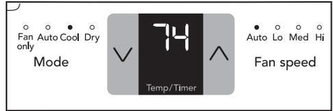
Note: Fan starts at Low Speed and adjusts to a proper speed according to the room temperature dictates. For example, if the room doesn't get too warm, it will stay at the slowest speed. If the room temperature rises quickly, such as a door being opened, it will automatically go to the highest speed. The fan speeds will re-adjust back to the slowest speed as the room returns to the original set temperature.
