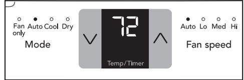
Note: This mode is a fixed combination of Cool mode and Auto fan speed setting. In this mode, the fan speed can not be selected manually.
