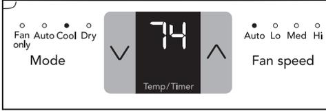
Note: Tap or hold either up (∧) or down (∨) button until the desired temperature is seen on the display. This temperature will be automatically maintained anywhere between 62 °F (17 °C) and 86 °F (30 °C). If you want the display to read the actual room temperature. See "To Operate on Fan Only" section.
