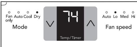
Note: In this mode, the air conditioner will work like a dehumidifier, but it will cool the room down meanwhile. The temperature can be adjusted between 62 °F (17 °C) and 86 °F (30 °C) and fan speed will be held at "Lo".
