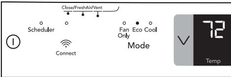
**NOTE: The unit will run in energy saver(econ) mode when powered on each time, if last shutdown is in cool or energy saver(econ) mode.** In this mode, the fan will continue to run for 3 minutes after compressor shuts off. The fan then cycles on for 90 seconds at 10 minute intervals until the room temperature is above the set temperature, at which time the compressor turns back on.
