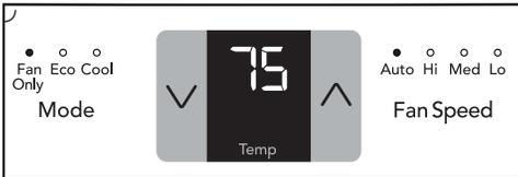
Note: Use this function only when cooling is not desired, such as for room air circulation or to exhaust stale air on some models. You can choose any fan speed you prefer. (Except "Auto Fan"). During this function, display will only show the actual room temperature and the set temperature can not be changed.
