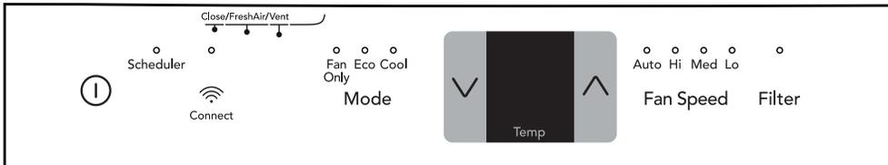
After 60 seconds of control inactivity the display and indicator lights will turn off. Press any button on the control panel or remote control and the display will resume. Please note that if the unit is in eco mode and the set temperature has been reached the unit may appear off. However, the unit is on and will continue to sample the air every 10 minutes. To confirm, press any button on the control panel or remote control to illuminate the display to show unit in eco mode.
