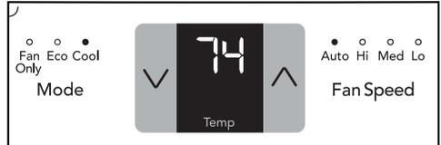
Note: In this mode, the fan remains on all the time with the compressor cycling on and off when room temperature is reached.
