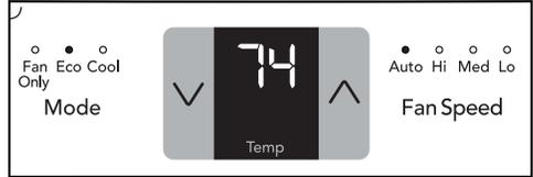
Note: The display will show the set temperature during normal operation, press either up (^) or down (v) button to adjust the set temperature to the desired setting. The unit will beep twice if the temperature up (^) or down (v) button is pressed continuously when the set temperature reaches the upper/lower limits 90°F or 60°F.
