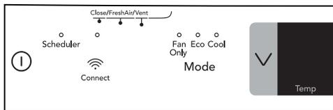
Note: After the unit is turned off, the light on the display will gradually fade away in 3 seconds. The unit will always return to “eco” mode and “auto” fan speed setting when it is turned on again.
