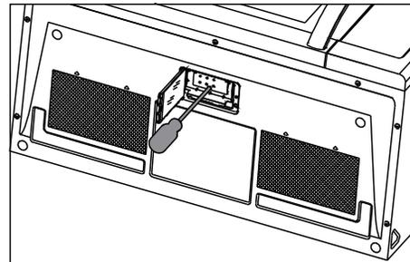
**Disconnect the power cord or leave the door open to deactivate the oven during cleaning. Disconnect the power cord before replacing filters and lights.**
