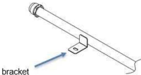
In case of replacement of the gas supply pipe, the spare part is supplied with the bracket shown in the figure to the side.
