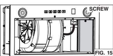
4. Punch out one of the two knock-out holes. Install an appropriate 7/8" diameter strain relief (not included, grey part in FIG. 16). NOTE: The HCK44 cord connection kit (optional) can be used instead of the house power cable. Refer to the instruction packed with the HCK44 cord connection kit.
