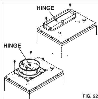
NOTE: The damper hinge must be towards the front of the unit.
