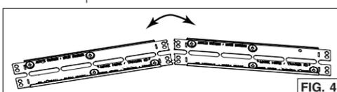
NOTE: Both cabinet brackets have one wide edge and one narrow edge (FIG. 5), to cover all installation configurations depending on cabinet widths.
