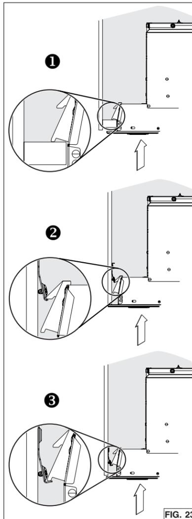
2. Insert the unit in the cabinet, until you feel a 'click' from both sides of the unit, confirming that the Ease of Install hooks rest on the top of the cabinet bottom sides 1, or cabinet brackets 2 or 3 (FIG. 23). Move the unit from left to right, from rear to front and up to ensure the Ease of Install hooks are retaining the unit inside the cabinet. NOTE: The unit will be protruding below the cabinetry until tightened.
