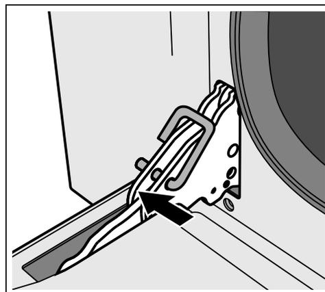
3. Close the oven door until it catches on the hinge stop levers, locking the hinges at the correct angle for door removal. The door can be removed when it is pulled up from the open position by about 8 inches (203 mm). This takes the tension off the spring-loaded hinges so that the door can be easily lifted out.
