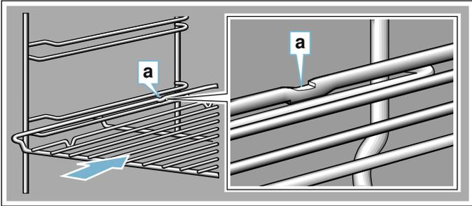
3. Tilt rack up to allow stop into rack guide.
