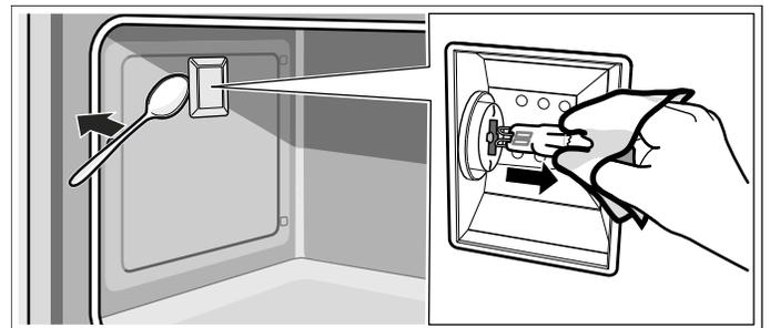
7. Replace the oven light bulb with a bulb of the same type.
