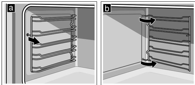
4. Replace the self-cleaning surfaces and rack guides in the reverse order in which they were removed.
