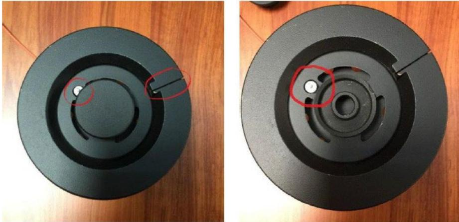
2. Make sure the electrode is going through the hole on the flame ring and it is **vertical to the surface of flame ring base**.
