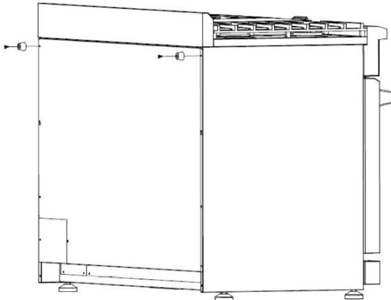
2. Install the 2 rubber pads as shown above.
