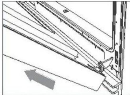
2. Fully open the levers on both sides.
