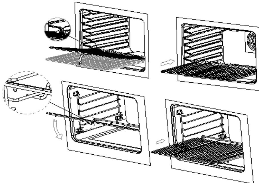
5. Lift the front about 15° upward till the tag of the shelf clears the safety stop of the side rack. Then lower the shelf horizontally and slide all the way into the oven. Other shelves can be installed this way.
