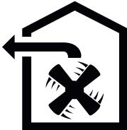
The air that is drawn in is cleaned by the grease filters and exhausted outdoors by a ductwork.
