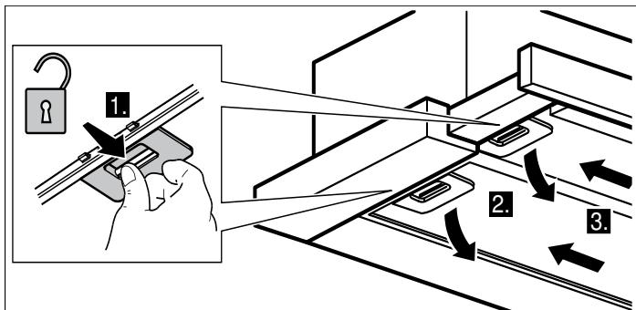
**Note:** Grease can accumulate in the bottom of the metal mesh grease filter. Do not hold metal mesh grease filter at an angle, otherwise grease will drip out.
