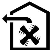
The air that is drawn in is cleaned by the grease filters and conveyed to the exterior by a pipe system.
