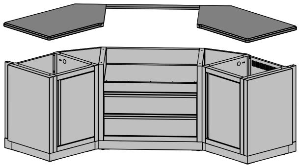
COUNTERTOP TO BE FASTENED AS PER MANUFACTURER'S INSTRUCTIONS. HOLES HAVE BEEN PLACED ON THE TOP FLANGE OF THE SIDE PANELS TO ALLOW FOR FASTENERS.
