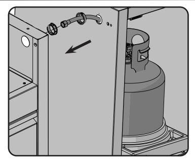
Knockouts have been punched in the sides and back panels to provide easy routing of gas or electrical piping. Once the knockout has been removed a bushing must be installed to prevent the gas or electrical line being cut on the edge of the hole. Gas piping and installation must be done by a qualified gas installer.
