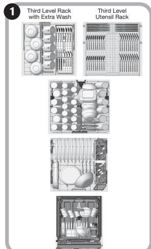
**Prepare and Load the Dishwasher** (14 Place Setting Recommended Loading Pattern)
