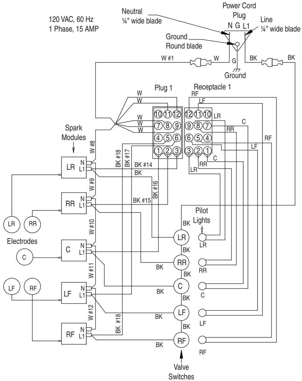
**NOTE:** Electric circuit is closed when knob is pushed in and rotated from 0° to 210° counterclockwise from Off.
