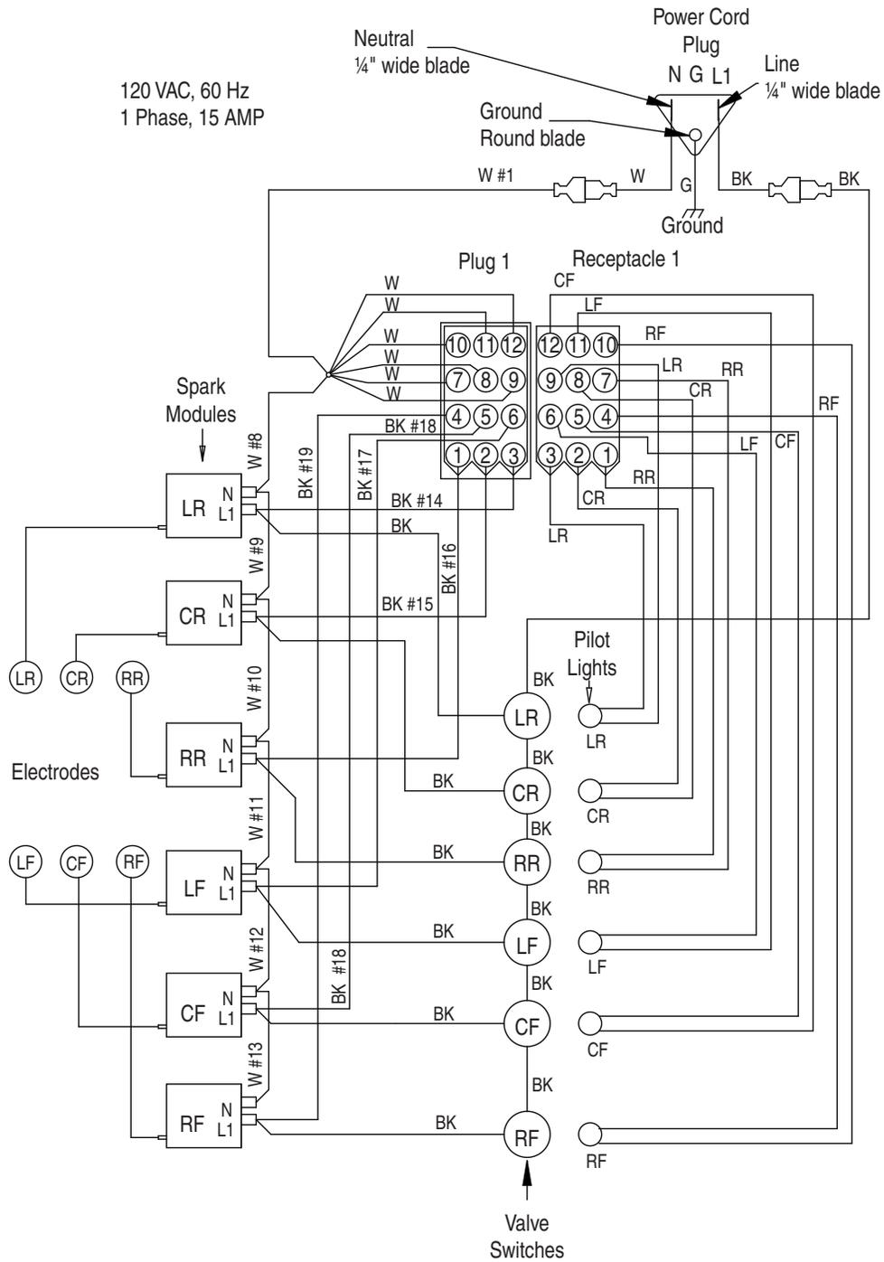
**NOTE:** Electric circuit is closed when knob is pushed in and rotated from 0° to 210° counterclockwise from Off.
