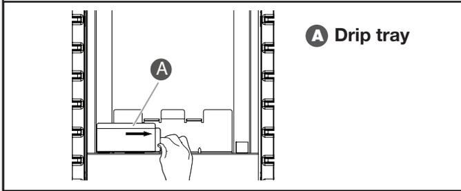
Slide drip tray into opening on the left front side of the grill basin.
