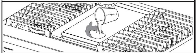
Using a measuring cup, pour up to 1 cup (236.6 mL) tap water over the soiled area. Start at the back, allowing the water to run toward the drip tray in the front. Allow the water to bubble on the griddle for 3–4 seconds.
