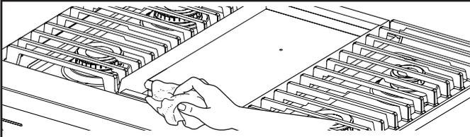
Clean the drip tray with warm, soapy water. Wipe the area under the drip tray clean. Once dry, put the drip tray back in position.
