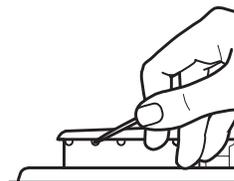
Use a straight pin. Do not enlarge or distort the port. Do not use a wooden toothpick. If the burner needs to be adjusted, contact a trained repair specialist.
