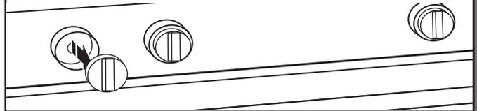
Pull the knobs straight away from the control panel to remove.
