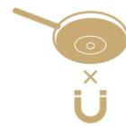
To determine if a pot is suitable, a magnet may be used to check whether pots are magnetic.
