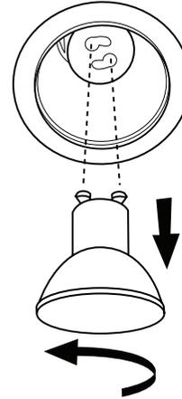
3. Remove the bulb and replace it with a 120 V, 50 watt maximum halogen bulb with a GU10 base. Turn it clockwise to lock it into place.
