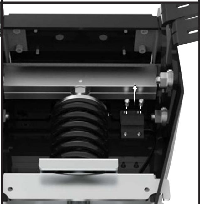
Remove the 2 screws from the upper half of the lid switch. (Note- DO NOT remove the top 2 screws from the mounting plate).
