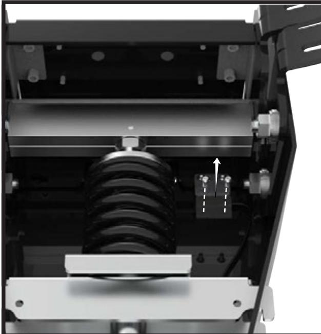
Remove the 2 screws from the lower half of the lid switch.
