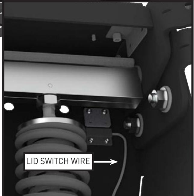
Repeat the steps in reverse order to install the new lid switch (Note - when reinstalling the lower half of the lid switch, make sure the wire goes towards the outside of the hinge).
