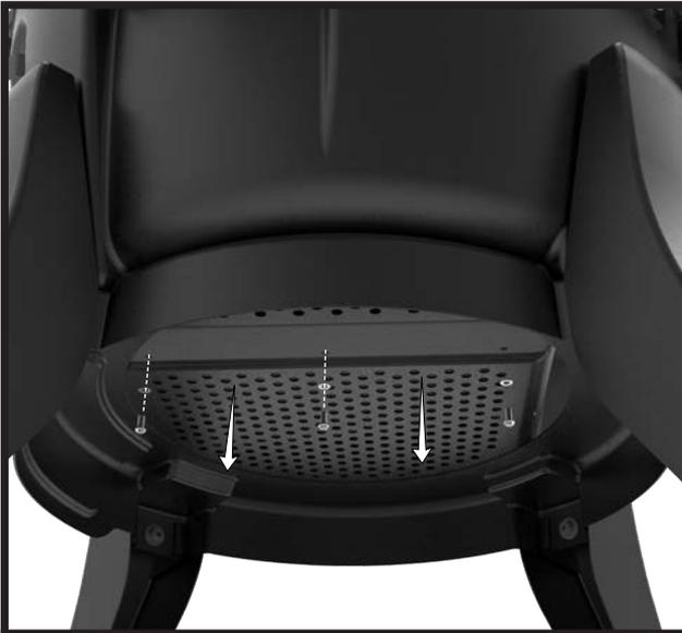
Remove the three wire harness cover screws.
