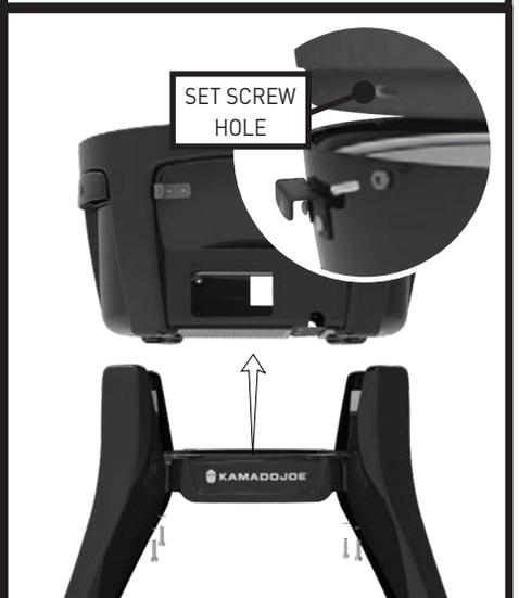
Remove the black base from the cart – remember to remove the 4 screws that connect the grill base to the cart. Note - when installing the ceramic base, line up the hole in the ceramic with the front set screw location on the grill.
