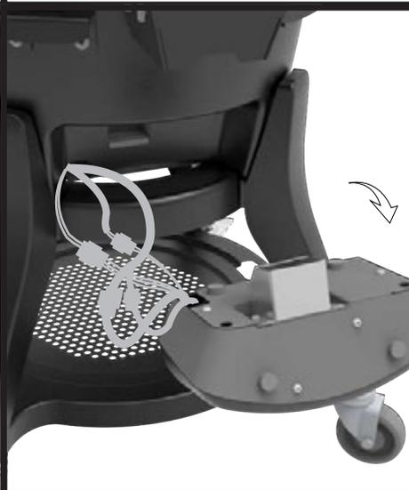
Disconnect the wire harness from the rear module. Use caution do not apply tension on the wire harness. Set the rear module aside, you will need to install this on the new black base kit.
