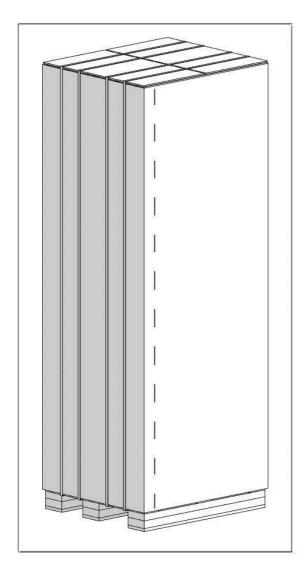
Remove the Packaging Polystyrene material.
