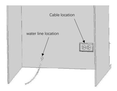
Method B : Locate the water hose and power supply on the side
