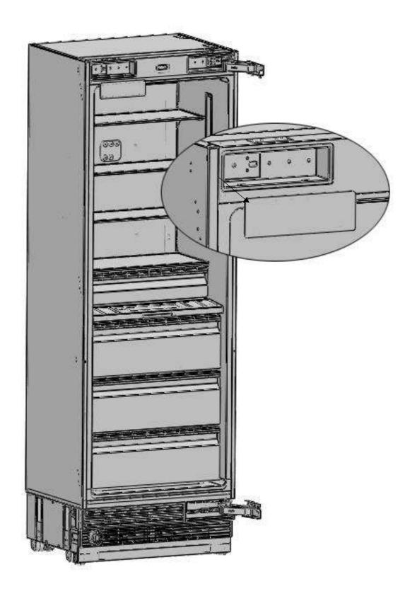
Remove the lower right hinge by loosening its 2 screws and fix it to its slot at the upper left side.
