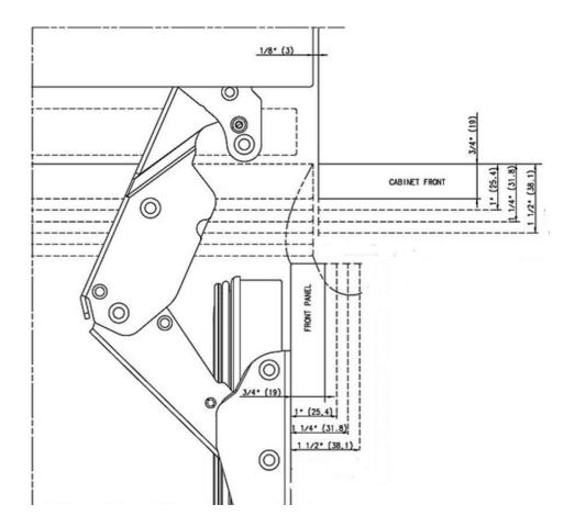
You can limit the opening degree of your door to  $90^\circ$  If you want  $90^\circ$  limit pin (item No.17) is located in the mouting part kit of the drawer box. Pin must be fully seated in the bracket or the door will not close properly.
