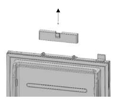
• Loosen screws of the lower cover of the door and remove it.
