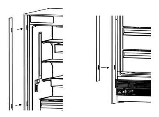
Attach the upper closing part onto the upper connection bracket.
