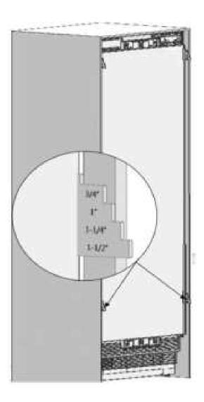
• Position of the level adjustment part (10) must be adjusted according to the thickness of the door. It can adjust the level for 4 different door thickness levels.
