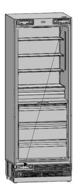
• Attach the Hinge Slot Caps removed from the left side to the Hinge Caps to the right side.
