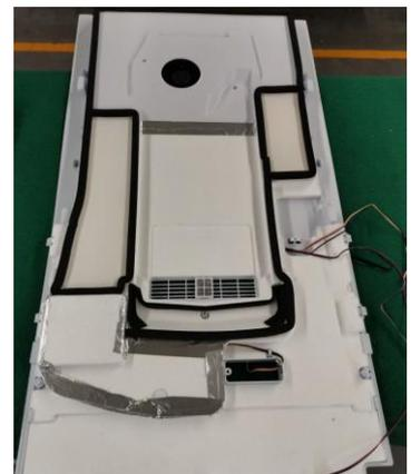
3. Remove the air duct coverplate
