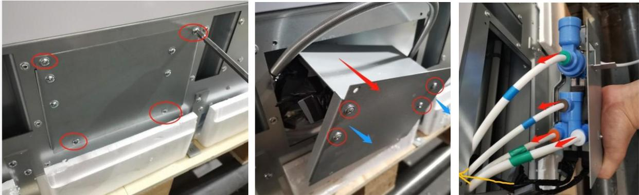
1. Remove the four screws securing the water valve from the side
