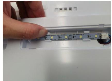
1. Icehouse light bar on the back of the display compartment
