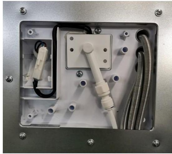
Fill Tube Heaters & Water Lines
