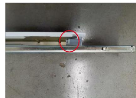
1. Removal of frozen lower rail set screws using tools 2. Circles are fixed with snaps
