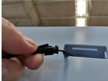
2. Press the connector self-locking catch to remove the magnetic switch
