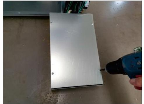
3. Remove the 2 screws that fix the main control board
