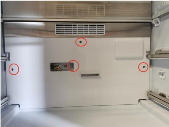
1. Remove the cover plate fixing screws
