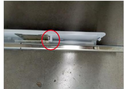
1. Removal of the freezing upper rail fixing screw using a tool 2. Circles are fixed with snaps
