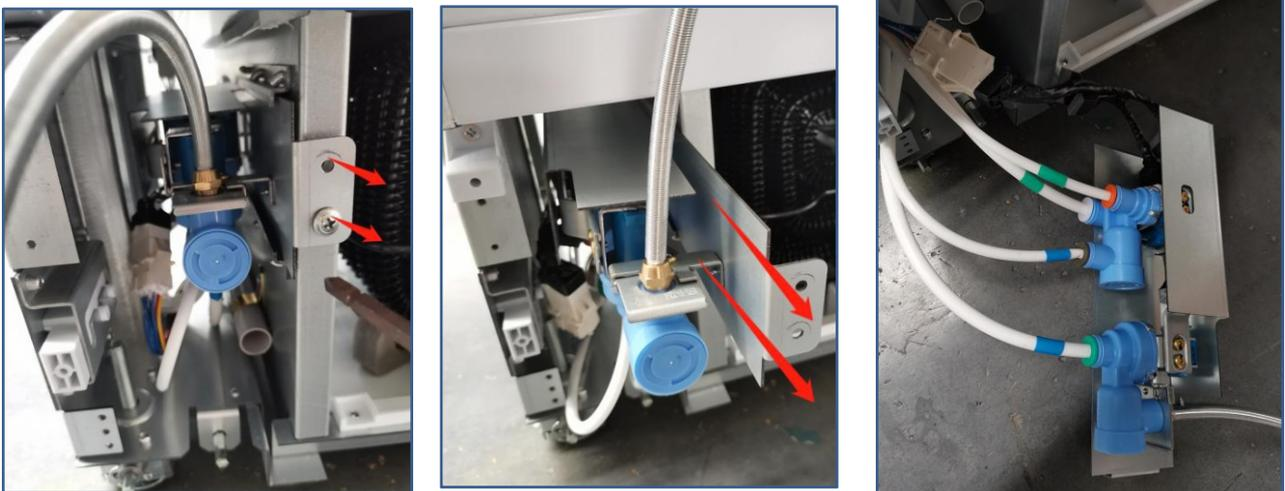
1. Remove the four screws securing the water valve from the front
