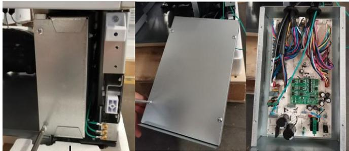
Control board repair from the lower right of the front
