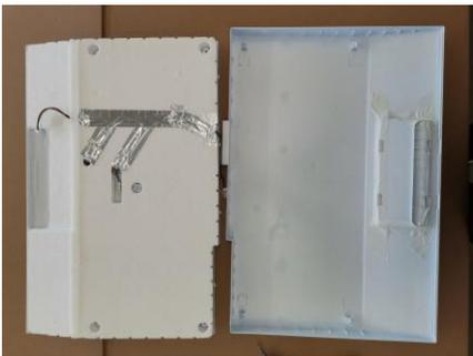
7. Open the top and bottom cover of the display panel and remove the protective cover tape of the display panel
