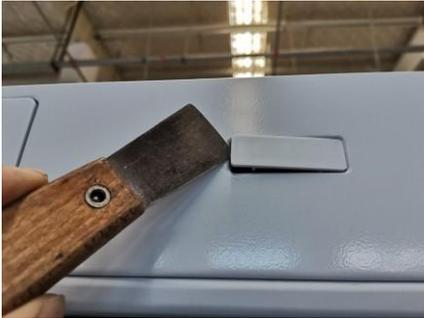
1. Use the flat shovel to pry open the magnetic switch box cover
