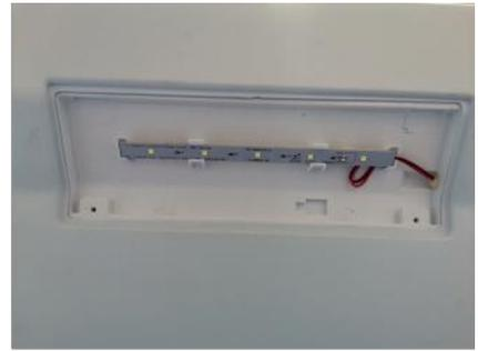
1. Use tools to remove the top light cover screws
