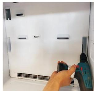
2. Remove the air duct fixing screws
