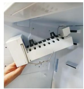
4. Unplug the terminals and remove the ice machine
