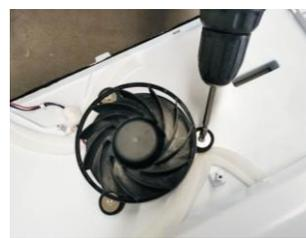
7. Removing the freezing fan
