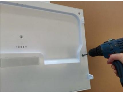
4. Remove the 5 screws on the back of the display partition
