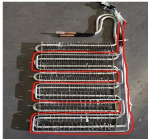
1. Pull out the freezer top drawer. Carefully pull forward on the evaporator to unclip it from the rear wall. Remove the two retaining clips from the front of the evaporator.
