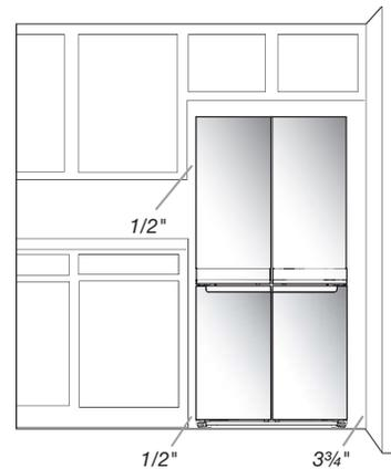
To ensure proper ventilation for your refrigerator, allow for a 1/2" (12.7 mm) space on each side and at the top. Allow for a 2" (50 mm) space behind the refrigerator. If your refrigerator has an ice maker, allow extra space at the back for the water line connections. When installing your refrigerator next to a fixed wall, leave a 3 3/4" (95 mm) minimum space between the refrigerator and wall to allow the door to swing open.
